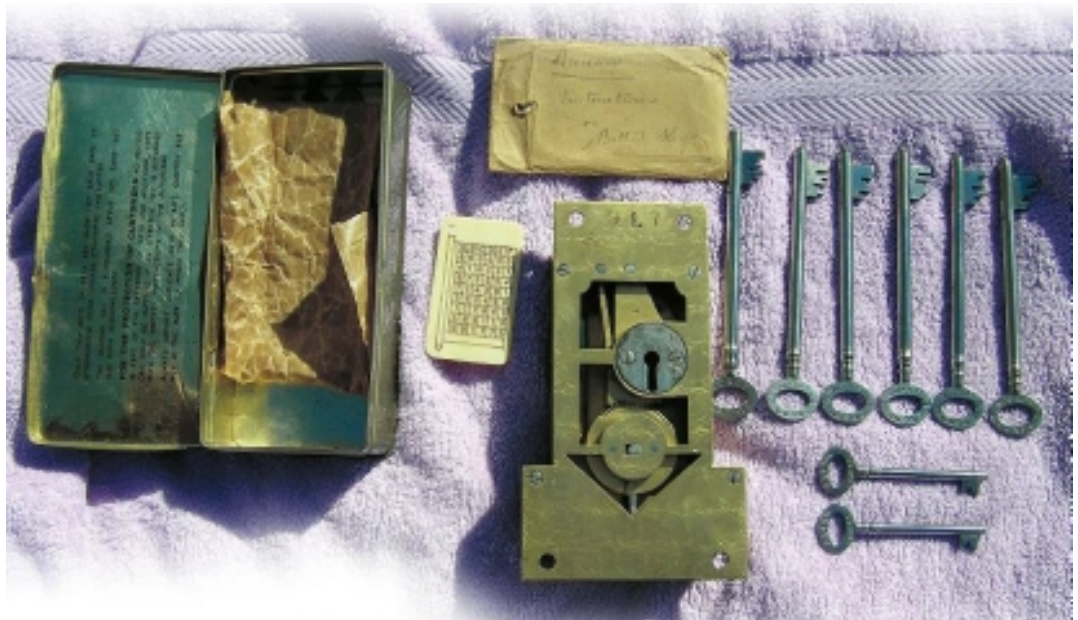
A lock set with original key tag marked days of the week, only 1 day key is missing. This set comes with 2 permutation keys (smallest keys) and 1 change key (with 7 removable steps). The lock has been nicely cutaway for demonstration purposes but it has not been finished to a display standard yet.
