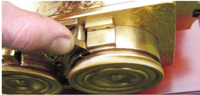
Depressing the curb security catch to unscrew the curb from the lock for maintenance.
