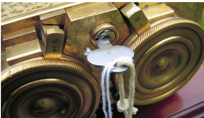
Both wheel curbs are secured each by a spring security catch. The spring catch is depressed to allow rotational movement of the curb to unscrew from the lock. For extra security the two catches can be locked preventing curb removal. This is by means of a dual control small lever lock, demonstrated with a set of steel flat keys, directly below in its open position. The dual control lock shoots a bolt plate to lock the Nickel control knobs in position. The Nickel control knobs allow modification of the lock by disengaging half of the lock mechanism, making a 5 wheel single dial, opposed to a 10 wheel double dial.
